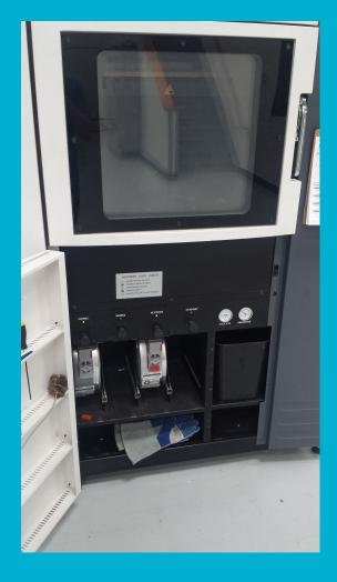
Bays for canisters. On the right side of the canister is an example of an open bay.
