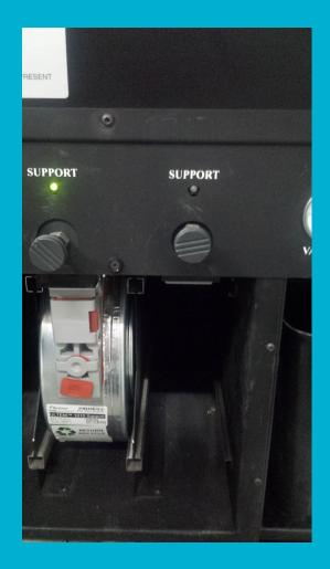
In an open bay section, the black metal inlet (material inlet) is used for inserting filaments.
